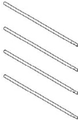
4 x pipe Ø25,4 x 1,0 mm L = 1000 mm, one end pressed
